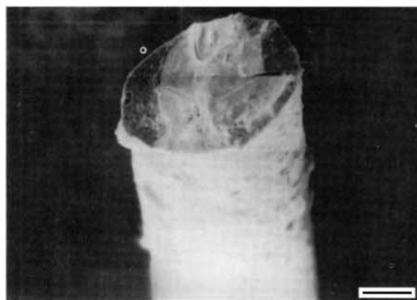
Figure 10 SEM micrograph of a tungsten glycolate/saccharose fibre annealed at 1200^\circ\text{C} (bar length 10\ \mu\text{m} ).
